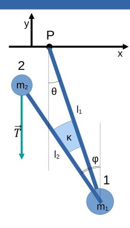
Let's suppose that a load is suspended to the device and that this load can be approximated with a constant vertical force.
